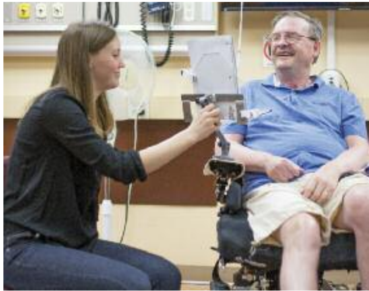
Janssen and Roud are prototyping a copy stand that can make holding a book and turning its pages easy enough for Stinson so he can read comfortably.
