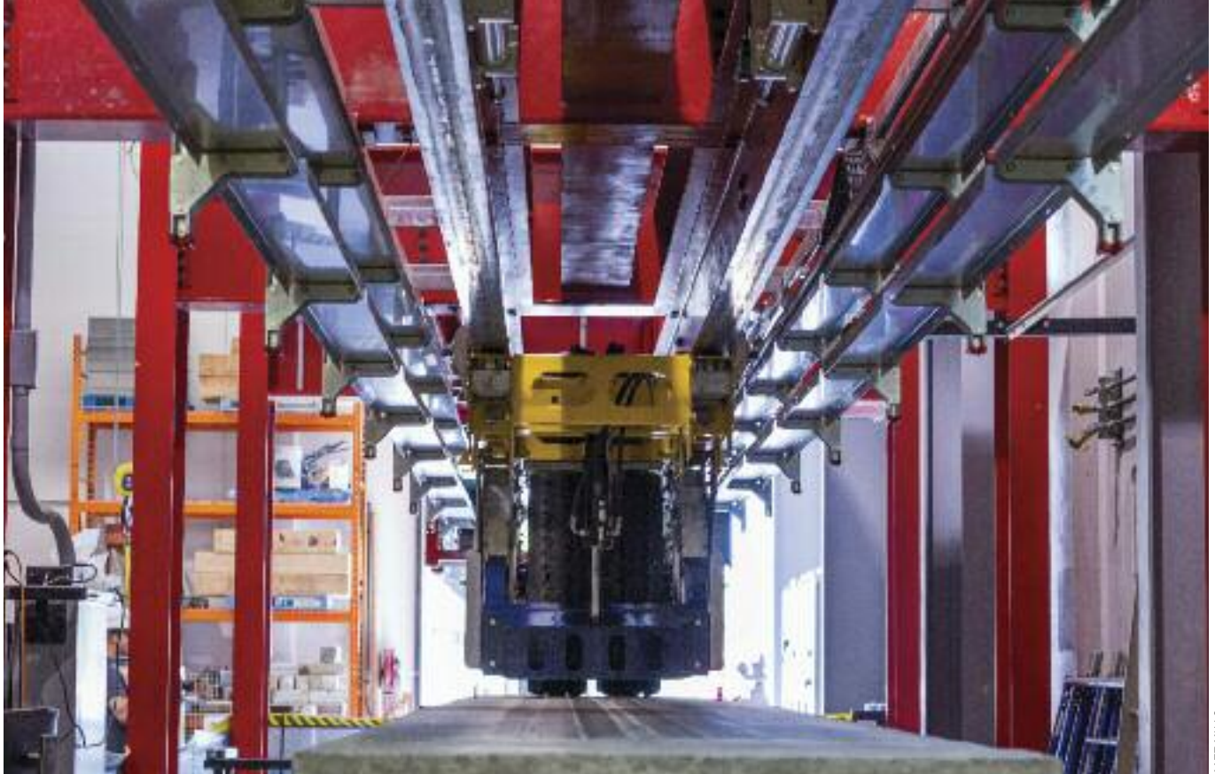
The Moving Load Simulator drives back and forth over a strip of test material, recreating the forces borne by a bridge.
