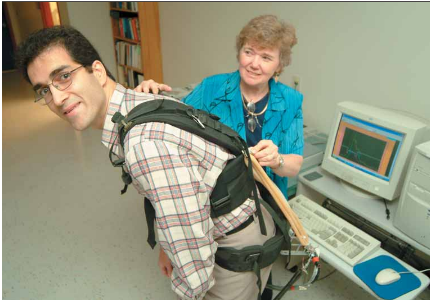
Joan Stevenson (Physical Education) adjusts settings on the PLAD (personal lift augmentation device) worn by PhD student Mohammad Abdoli, in Queen's Ergonomics Research Laboratory.
